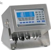
three axle weights and a gross weight. As soon as motion ceases on the scale it will automatically send all four readings to a printer or computer.
