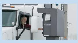
**Unattended Systems** Allows 24/7 scale availability. Can be customized with several hardware options such as loop detectors, ID readers, video surveillance, traffic lights, and wireless communication.
