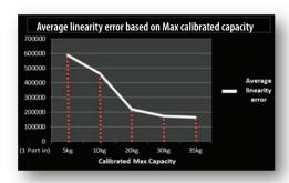
Linearity is measured from zero to calibrated max capacity. Hysteresis is measured from max capacity back to zero.
