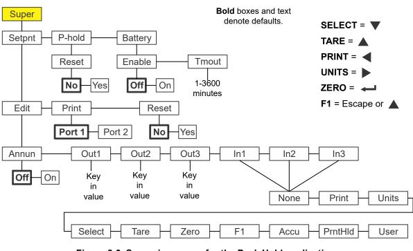
Figure 8.6 shows the Supervisor menu when you are in the Peak Hold application:
