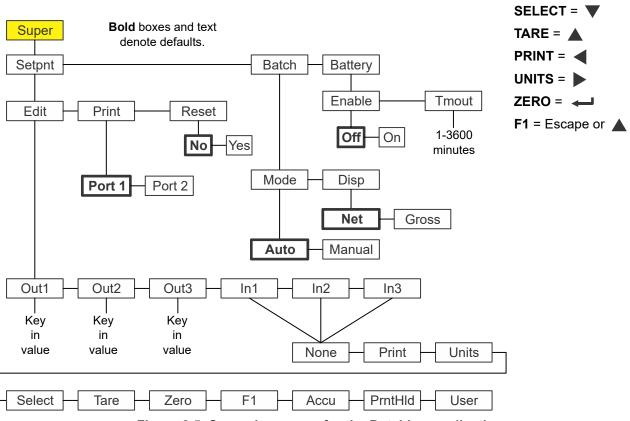
Figure 8.5 shows the Supervisor menu when you are in the Batching application:
