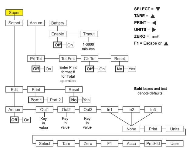
Figure 8.2 shows the Supervisor menu when you are in the Accumulator application:
