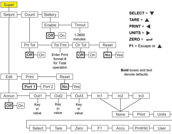
Figure 8.3 shows the Supervisor menu when you are in the Counting application:
