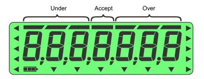
Figure 3.1 Checkweighing bargraph
