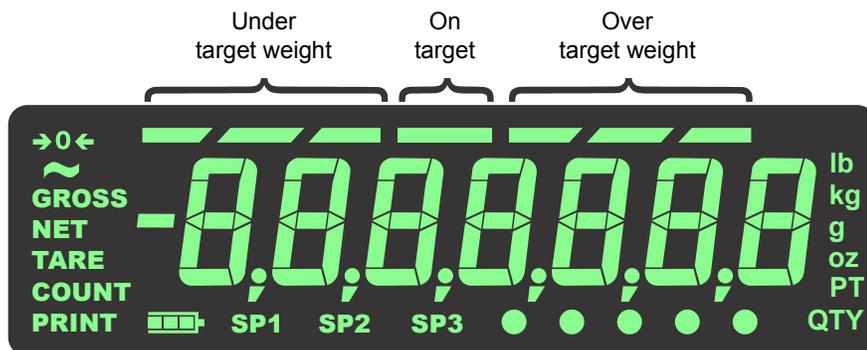
Figure 3.2 Checkweighing bargraph
