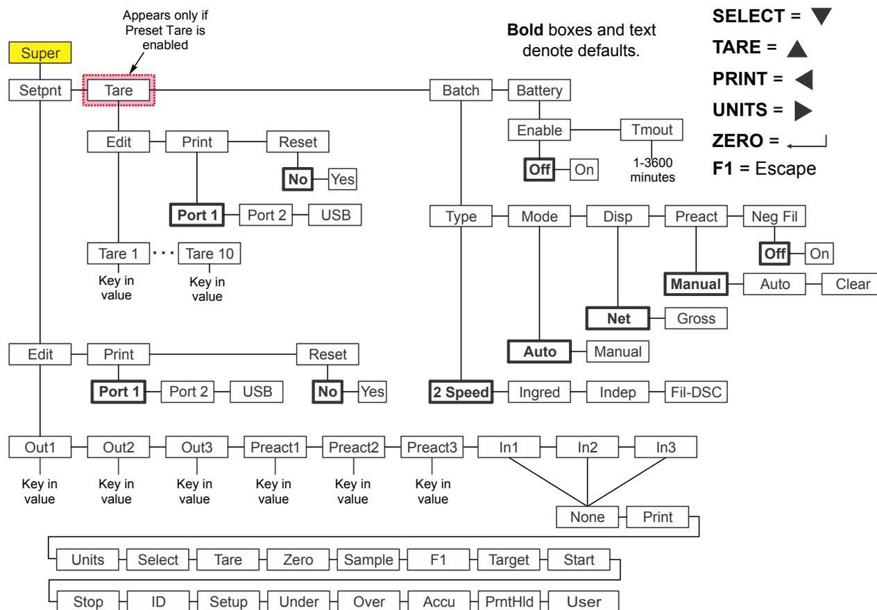
Figure 7.5 Supervisor menu for the Batching application
