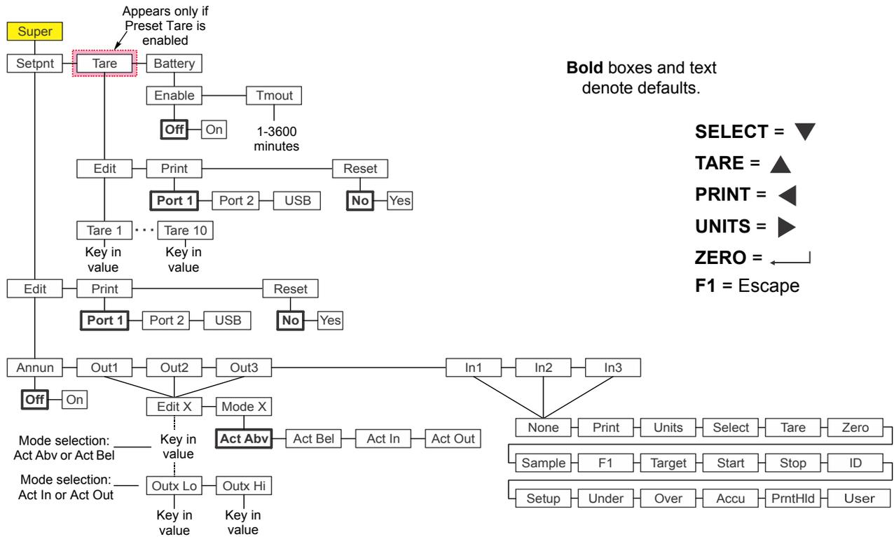
Figure 7.1 Supervisor menu for the General Weighing application
