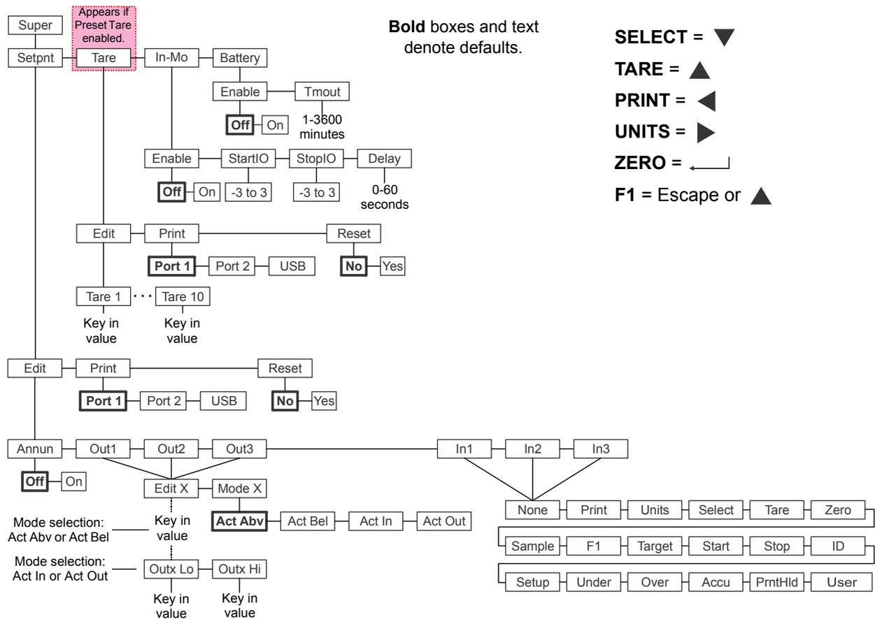
Figure 7.8 Supervisor menu for the In-Motion application
