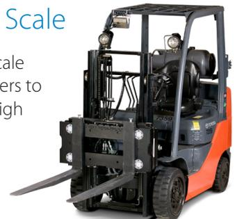
Optional in-cab instruments such as bar code scanners allow forklift operators to instantly capture all necessary freight data available and then transmit this information with weight data wirelessly via Bluetooth® or radio to supervisory computer systems.
