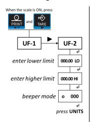
i. When the scale is ON, press **PRINT** and **TARE** keys together;
