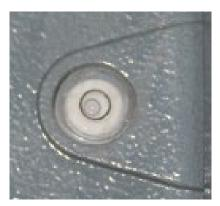
Fig. 2 Adjust feet until bubble is centered in the black circle
