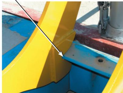
4. Be sure the safety tab slides down past the outside face of the outer Weigh Bar support plate as shown in the photos on the next page. This prevents the jacking frame from disengaging from the cover bolt plate.
