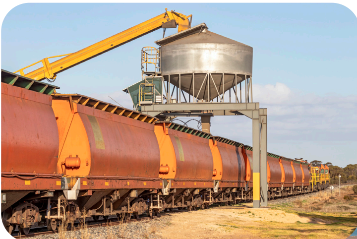
Grain weighing for bulk loading of trains
