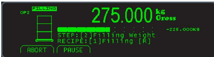
Weighing process bar showing the filling in progress and the amount still to be filled
