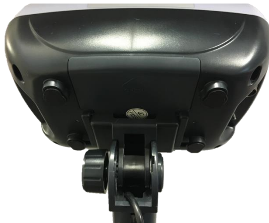
Fig. 4 Slide indicator head onto column bracket
