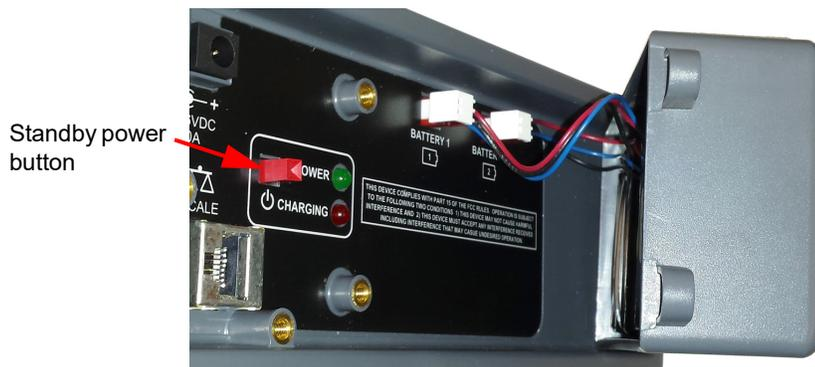
**Figure 2.8 Battery pack connections**
