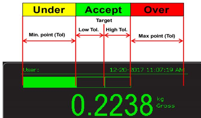
Figure 3.1 Tolerance mode
