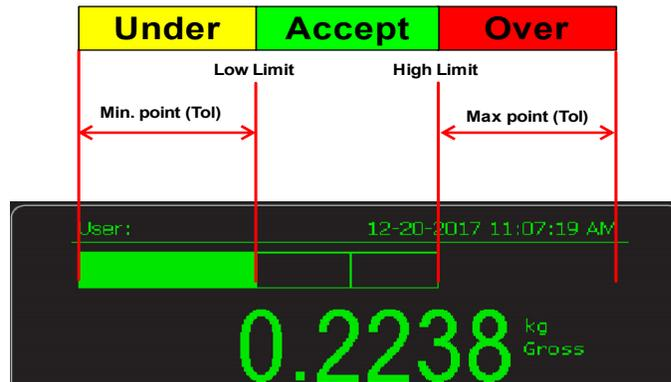
Figure 3.2 Tolerance mode
