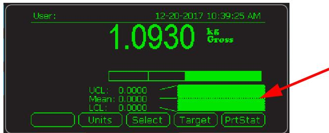
The graph, pointed out in the illustration above, shows the result of a rolling average of the last 100 (default) weighments. This displays the average weight reading along with the highest & lowest recorded weight seen in that buffer window. You can set the number of weighments being averaged from 5 to 1000. A visual line shows you if the average is above or below the current target point.
