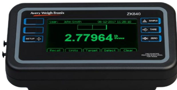
Checkweighing screen showing over weight
