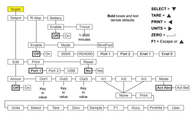
Figure 7.7 Supervisor menu for the Remote Display application
