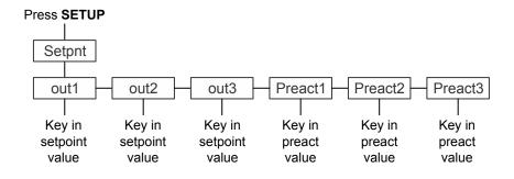
Setpoint or Preact values can be either positive or negative, up to or equal to scale capacity. See *Entering a negative number on page 15* on how to enter negative values.
