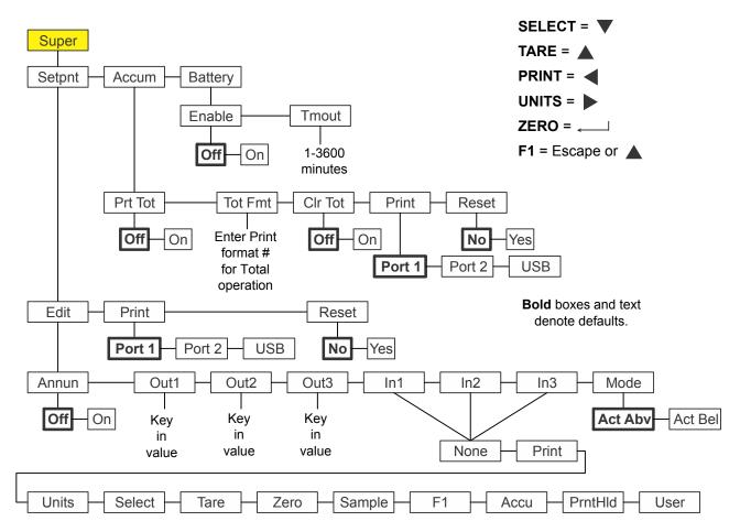
Figure 7.2 Supervisor menu for the Accumulator application
