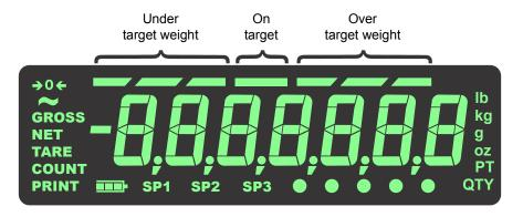
Figure 3.1 Checkweighing bargraph
