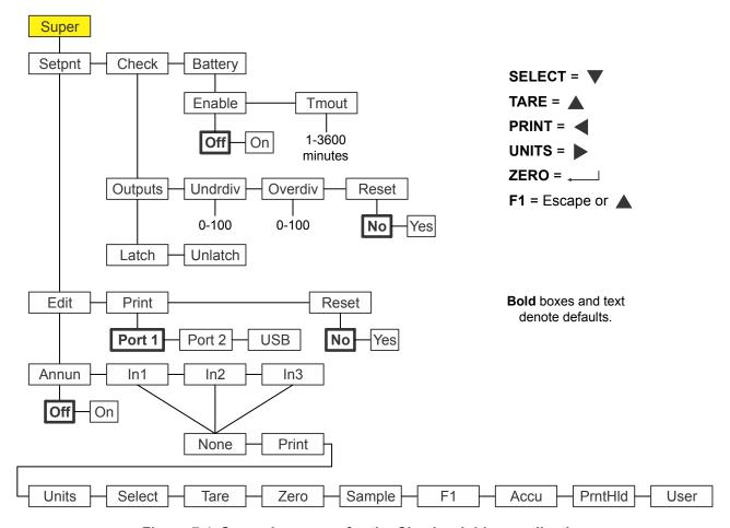
Figure 7.4 Supervisor menu for the Checkweighing application
