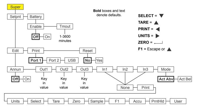
Figure 7.1 Supervisor menu for the General Weighing application
