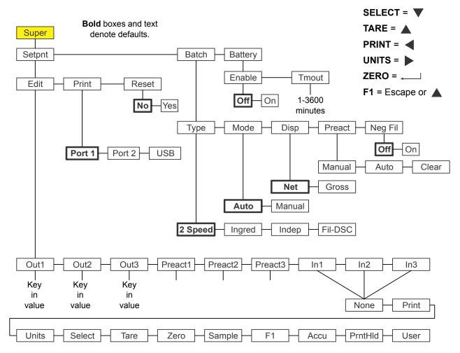
Figure 7.5 Supervisor menu for the Batching application
