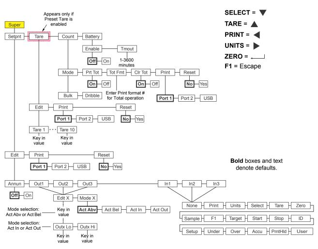
Figure 7.3 shows the Supervisor menu when you are in the Counting application:
