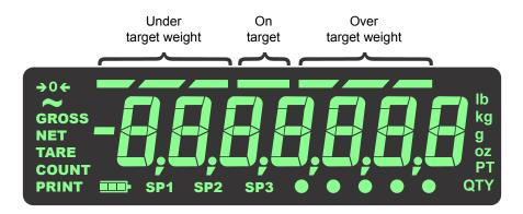
Figure 3.2 Checkweighing bargraph
