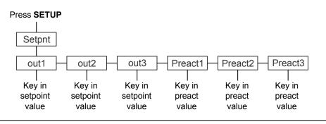
Setpoint or Preact values can be either positive or negative, up to or equal to scale capacity. See *Entering a negative number on page 14* on how to enter negative values.
