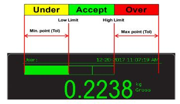
Figure 3.2 Tolerance mode
