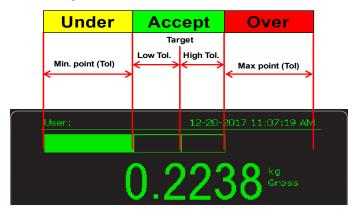
Figure 3.1 Tolerance mode
