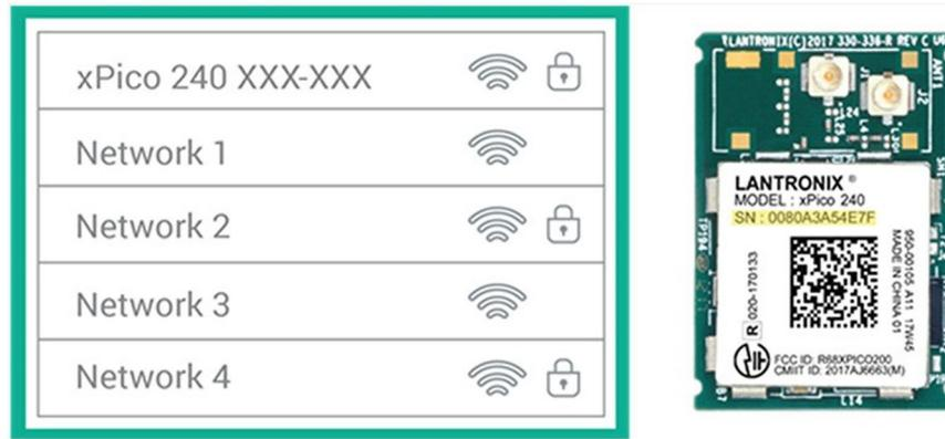
3. In a web browser, go to **192.168.0.1**. This is the default IP address when the module is an access point (AP). This will take you to a login page that is hosted by the module. These are the default credentials to log in (both are case sensitive):
