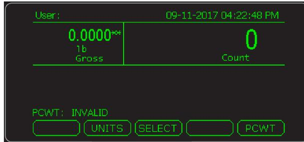
The Count application without the database is active by default. The screen shows the user name and time and date in the top line. Below that is the current weight and the count screen. Below that are the piece weight and active softkeys.
