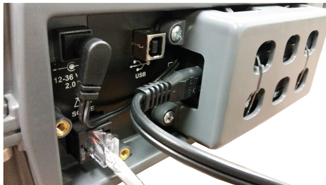
Figure 2.5 AC power connections
