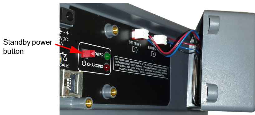
Figure 2.6 Battery pack connections
