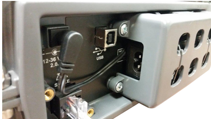
Figure 2.4 AC power block
