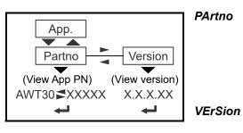
Use this to view the App part number. The part number is displayed in two parts. Press **RIGHT arrow** key or **LEFT arrow** key to toggle the display between the first and second parts of the part number.
