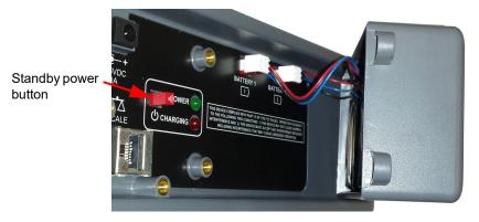
Figure 2.8 Battery pack connections
