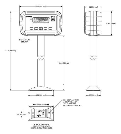
Figure 8.6 Pole mount and indicator dimensions
