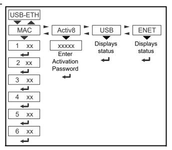
**uSb-Eth** The Ethernet and USB ports on the ZP900 are not functional unless activated. This menu contains information necessary to activate the two USB-HID and/or Ethernet ports on the ZP900. Record the MAC address found in this menu before contacting AWTX for activation code instructions.
