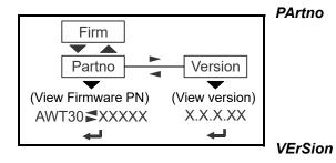
Use this to view the firmware part number. The part number is displayed in two parts. Press **RIGHT arrow** key or **LEFT arrow** key to toggle the display between the first and second parts of the part number.
