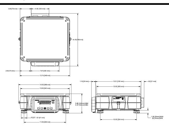
Figure 8.4 Model 1214 BSQ dimensions with PSU and indicator
