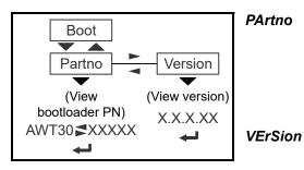
Use this to view the bootloader part number. The part number is displayed in two parts. Press **RIGHT arrow** key or **LEFT arrow** key to toggle the display between the first and second parts of the part number.
