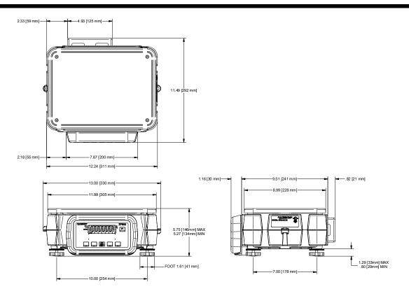
Figure 8.2 Model 0912 BSQ dimensions with PSU and indicator
