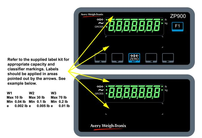
The front panels for the ZP900 indicator and remote display are shown in Figure 2.9 and consists of the keys and the display.
