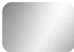
Fine brushed finish to Ra 0.8 \mu\text{m} is preferred
