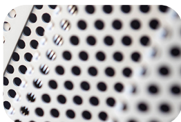
Not preferred due to being impossible to fully clean
