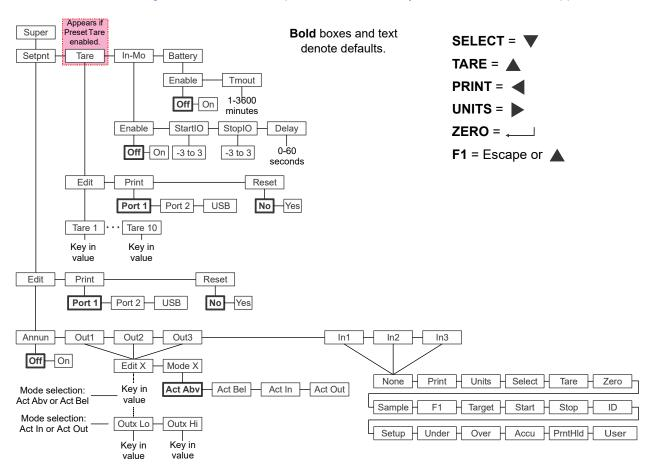
Figure 7.8 shows the Supervisor menu when you are in the In-Motion application:
