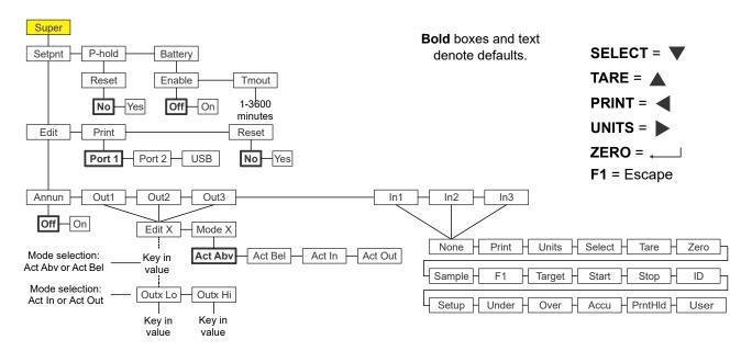
Figure 7.6 shows the Supervisor menu when you are in the Peak Hold application:
