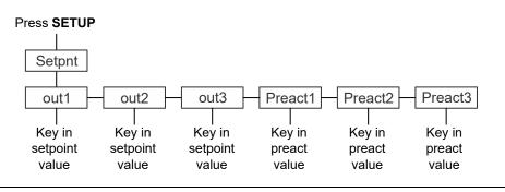
Setpoint or Preact values can be either positive or negative, up to or equal to scale capacity. See *Entering a negative number on page 12* on how to enter negative values.
