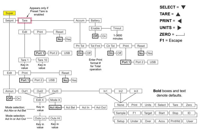
Figure 7.2 shows the Supervisor menu when you are in the Accumulator application:
