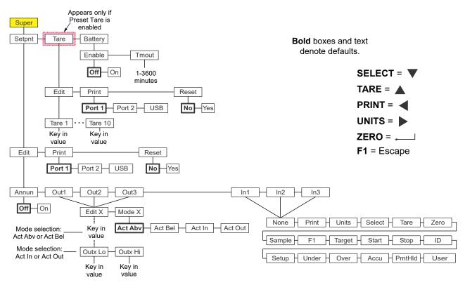
Figure 7.1 shows the Supervisor menu when you are in the General Weighing application.
