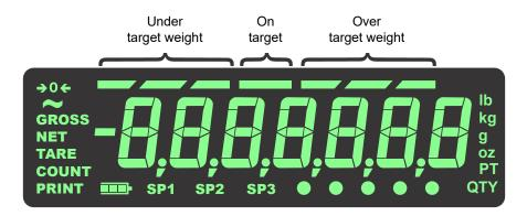
Figure 3.2 Checkweighing bargraph
