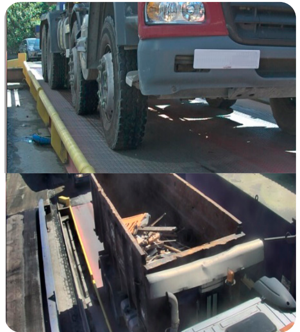
Vehicle positioning and overhead cameras capture images to be stored in Weighman8
