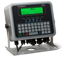
**ZM510** – A dot matrix 320 x 80 display can be used to create personalized messages such as user prompts, images and status annunciators. (Inverted display colors shown). A large QWERTY keypad offers input flexibility where adding an external keyboard would be difficult, such as panel-mount applications.
