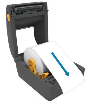
Pull the end of the roll past the front edge of the printer.
