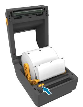
Align the sensor to the edge of the roll for marked labels.
