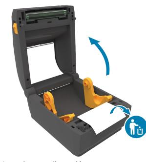
Open the printer and remove the packing.
