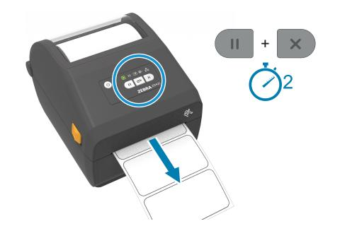
Press and hold the **Pause** and **Cancel** buttons for two seconds to line up the labels.
