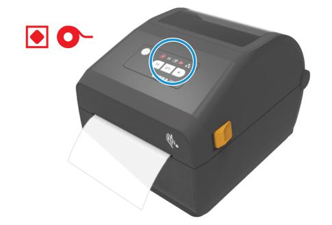
When the the printer is ready, the printer status light will turn green.
