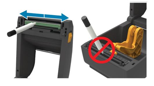
Clean printhead with a cleaning pen. Clean from the middle to the outside. Do not use a cleaning pen on the platen.
