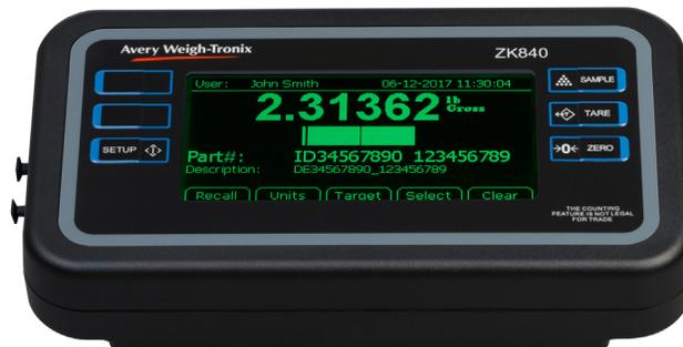
Checkweighing screen showing accept weight + PLU Database
