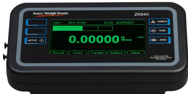
Checkweighing screen showing under weight
